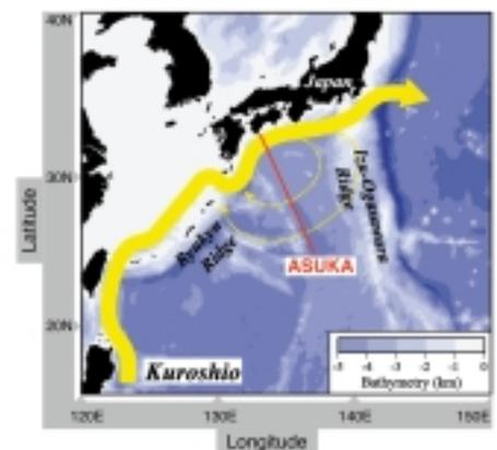
**Figure 1: ASUKA observational line (red line) across the Kuroshio south of Japan, superimposed on the bathymetry. Moored current meter measurements, repeated hydrographic surveys and other measurements were carried out on the line from October 1993 to November 1995. This line was purposely located along a track of the TOPEX/POSEIDON altimeter. Schematic flow patterns of the Kuroshio and its recirculation south of Japan are also shown.**
