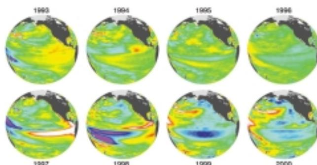
**Figure 1: Yearly Averaged Ocean Topography of the Pacific Ocean from the T/P data 1993-2000. See the high sea level expansion (in white), created by the 97 El Niño, along the east equatorial Pacific which is replaced in 98-99 by La Nina negative anomaly (in blue) (Courtesy of NASA’s Jet Propulsion Laboratory.)**
