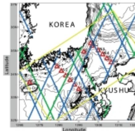
**Figure 1: The position of the in-situ ADCP and PG instruments, T/P ground tracks (green), Geosat ground tracks (blue), and the domain of the local adjoint assimilation model. The model will be used to form a solution that minimizes the difference to dynamical equations, the in-situ measurements, and altimeter sea level variations.**
