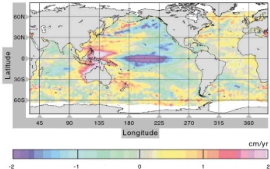
**Figure 2:** Sea level trends from the TOPEX/POSEIDON mission from linear regression analysis using eight years of satellite data. Jason-1 and future satellites are needed to study the effects on climate changes on sea level.
