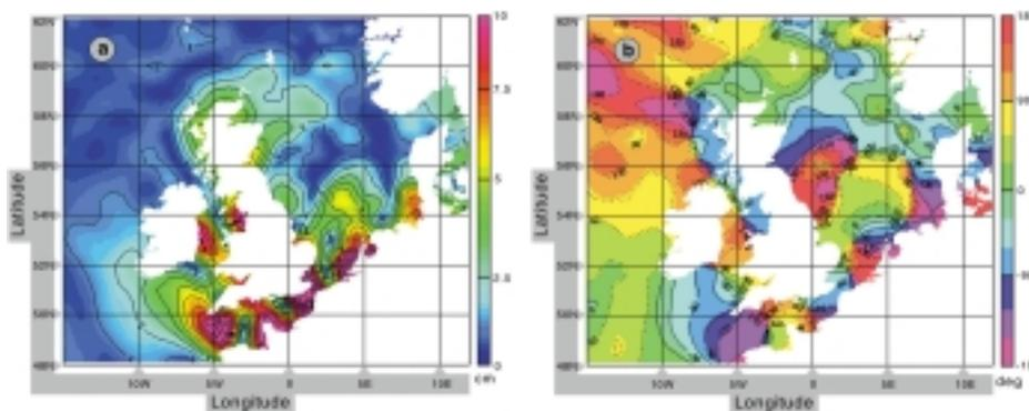
**Figure 1: Ocean tide models have been improved in shallow water regions using TOPEX/POSEIDON altimetry. In the North Sea the M4 tidal constituent, which has a period of about six hours, is considerable. The proposed tandem mission of Jason-1 and TOPEX/POSEIDON (interleaved ground tracks) will provide a unique opportunity to improve on those models. a) Amplitude in centimetres, b) Phase in degrees.**
