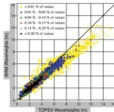
**Figure 3: Comparison of  $H_{1/3}$  data derived from a global model (WAM) and from TOPEX/POSEIDON.**
