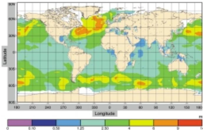
**Figure 1: Wave field ( $H_{1/3}$ ) calculated by Météo-France's VAG global model.**
