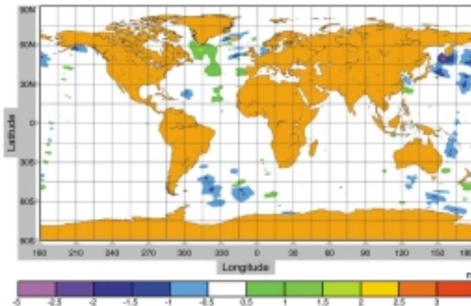
**Figure 2: Corrections to initial data (analysis increments) calculated by wave model from ERS-2 altimetry data for March 8, 2001 at 00.00 UTC. Only corrections larger than 0.5 meters are shown.**
