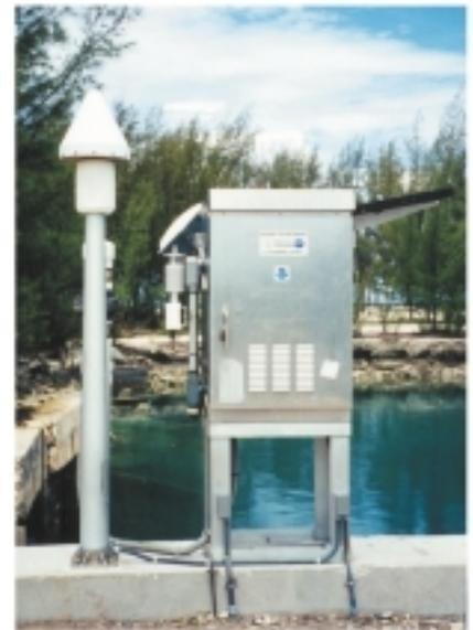
Figure 2: CGPS@tide gauge installation at Settlement Point, Bahamas. The GPS receiver is to the triangular shaped object to the left of the picture. The acoustic tide gauge sensor is directly behind the GPS monument.
