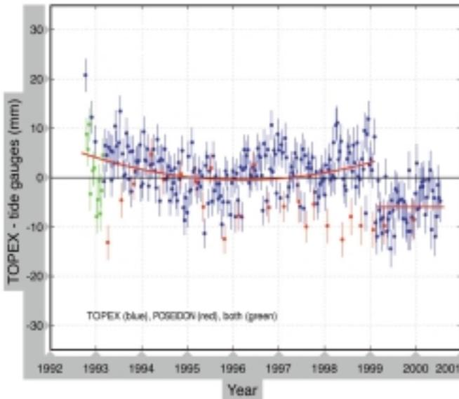
**Figure 1: 10 day estimates TOPEX and POSEIDON altimeter calibration estimates computed from altimeter minus tide gauge sea level differences [Mitchum, 1994; 1998; 2000].**
