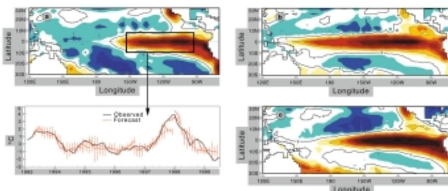
**Figure 2:** Example prediction of tropical ocean temperature anomalies over the TOPEX/POSEIDON period at CERFACS. Series of five six-month predictions, using a coupled ocean-atmosphere model, were carried out every three months. They show the model's ability to predict the 1997 El Niño event. (a) shows observations, (b) six-month and (c) three-month forecasts.
