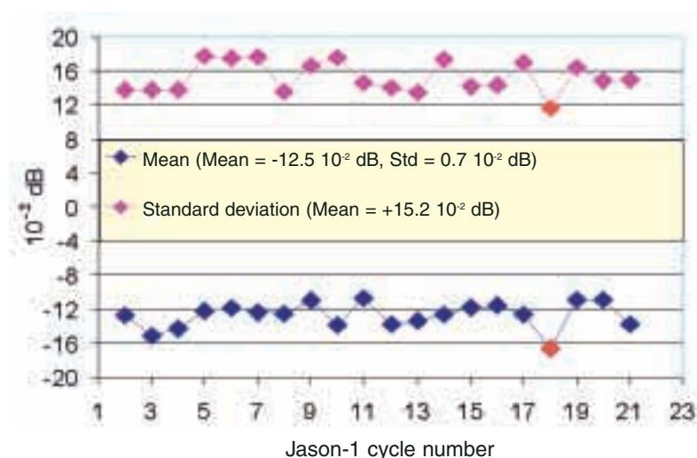
**Figure 1. Mean and RMS of sigma0 differences between Topex/Poseidon and Jason-1 (Units are dB) (On the “Mean” curve, blue diamonds are Topex measurements ,while the red one refers to Poseidon-I )**
