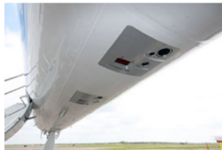
The MASS instrument was installed to make use of G-V nadir portals.
