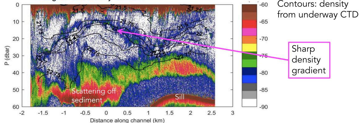
Acoustic data could capture MLD at ~1 m horizontal resolution
