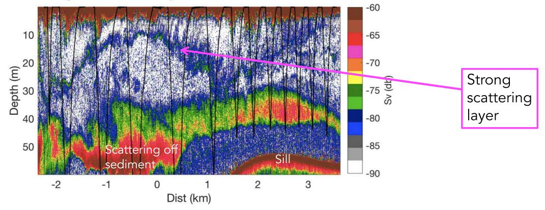
High-resolution mixed-layer depth & mixing from an acoustic echosounder (2017 Hood Canal Experiment)
