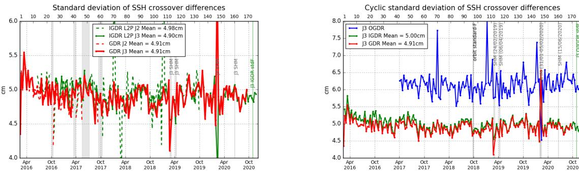
Figure 50 – Cycle by cycle standard deviation of SSH crossover differences for Jason-2 and Jason-3 (left), and for Jason-3 using OGDRs, IGDRs and GDRs (right). Only data with  $|latitude| < 50^\circ$ , bathymetry  $< -1000m$  and low oceanic variability were selected.
