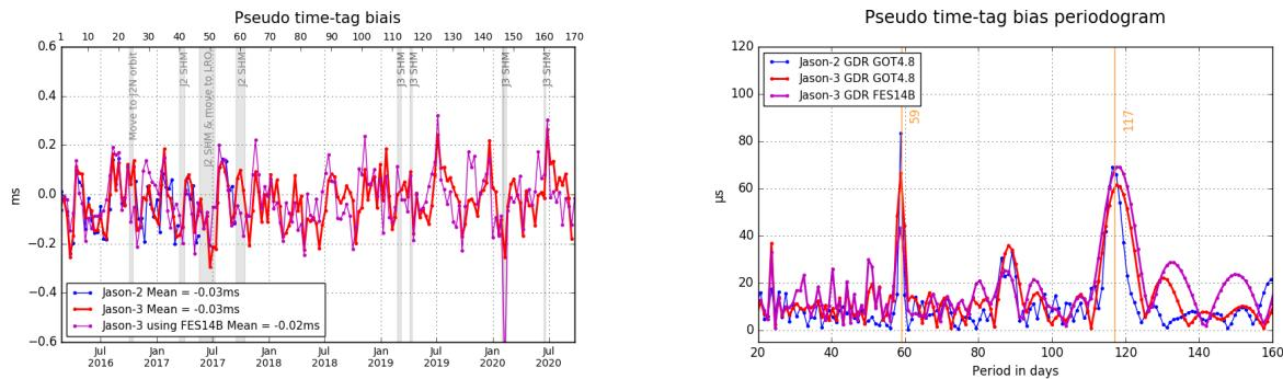
Figure 51 – Monitoring (left) and periodogram (right) of pseudo time-tag bias estimated cycle by cycle from GDR products for Jason-2 and Jason-3
