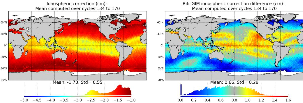
Figure 36 – Left: Map of ionospheric correction for Jason-3 averaged over cycles 134 to 170. Right: Map of dual-frequency minus GIM ionospheric correction solutions.
