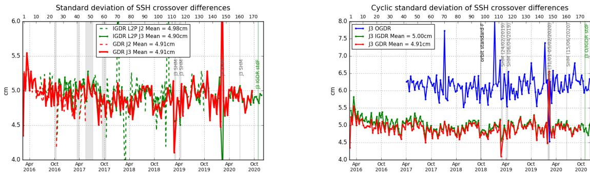
Figure 5 – Cycle by cycle standard deviation of SSH crossover differences for Jason-2 and Jason-3 (left), and for Jason-3 using OGDRs, IGDRs and GDRs (right). Only data with  $|\text{latitude}| < 50^\circ$ , bathymetry  $< -1000\text{m}$  and low oceanic variability were selected.
