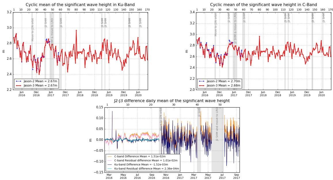
Figure 33 – Cyclic monitoring of significant wave height for Jason-2 and Jason-3 for Ku-band (left) and for C-band (right). Jason-2 - Jason-3 difference daily monitoring of significant wave height (bottom).
