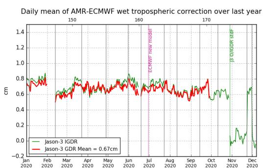
Figure 39 – Daily monitoring of AMR minus ECMWF model wet tropospheric correction over one year.
