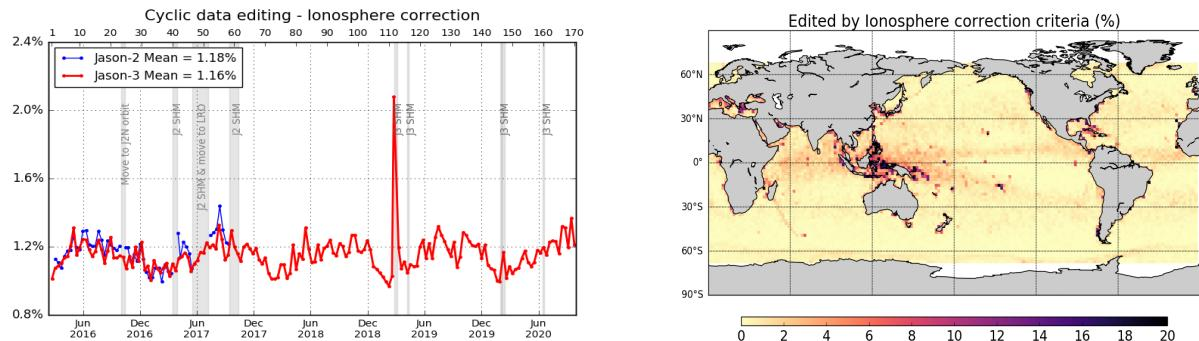
Figure 15 – Percentage of edited measurements by ionospheric correction threshold criterion. Left: Cycle per cycle monitoring compared with Jason-2. Right: Jason-3 averaged map from cycle 134 to 170.
