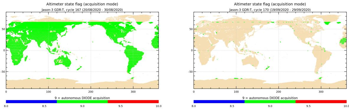
Figure 61 – Close loop coverage over OLTC v3 on the left (cycle 167) against OLTC v4 on the right (cycle 170)
