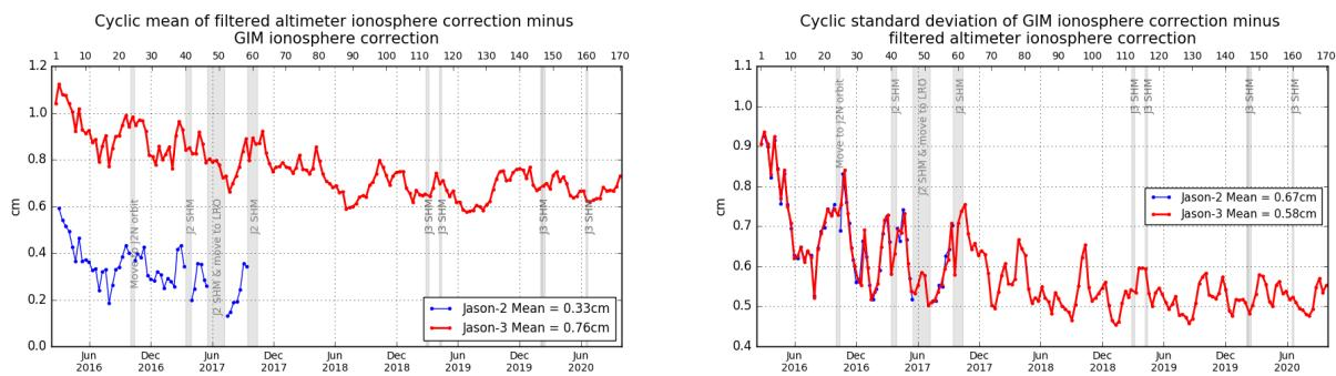
Figure 37 – Cyclic monitoring of GIM ionosphere correction minus filtered altimeter ionosphere correction for Jason-2 and Jason-3. Left: mean, right: standard deviation.
