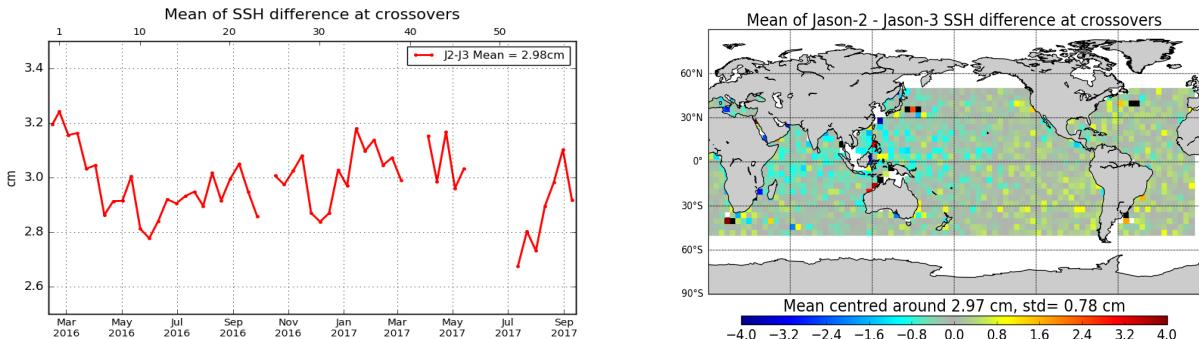
*Figure 49 – Cyclic monitoring of Jason-2 - Jason-3 SSH crossover differences mean (left) and map over cycle 1 to 58 (right). Only data with  $|latitude| < 50^\circ$ , bathymetry  $< -1000m$  and low oceanic variability were selected.*
