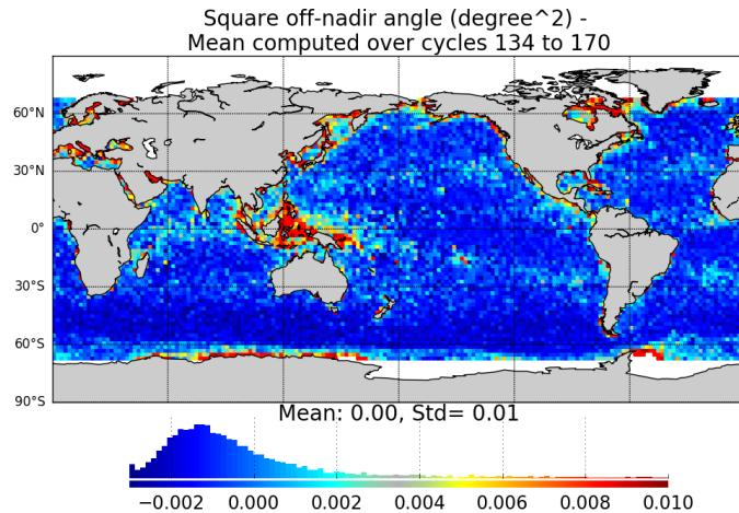
*Figure 27 – Map of the square off-nadir angle for Jason-3 averaged over cycles 134 to 170.*
