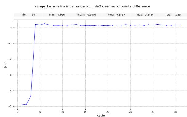
Figure 56 – Jason-3 GDRs : impact of MLE retracking on range computation over the first year
