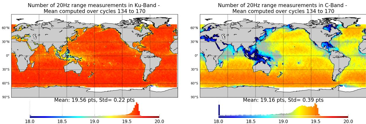
Figure 23 – Map of number of 20 Hz range measurements for Jason-3 averaged over cycles 134 to 170, in Ku-band (left) and in C-band (right).
