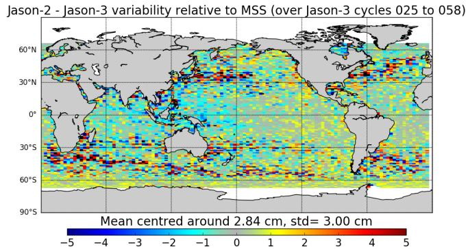
Figure 3 – GDR data. Map of Jason-2 and Jason-3 SLA differences for Jason-3 cycles 025 to 058
