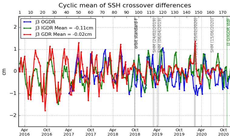
Figure 47 – Monitoring of mean of Jason-3 SSH crossover differences for OGDRs, IGDRs and GDRs. Only data with  $|latitude| < 50^\circ$ , bathymetry  $< -1000m$  and low oceanic variability were selected. (ocean\_tide\_sol1 = GOT is used in SSH computation)
