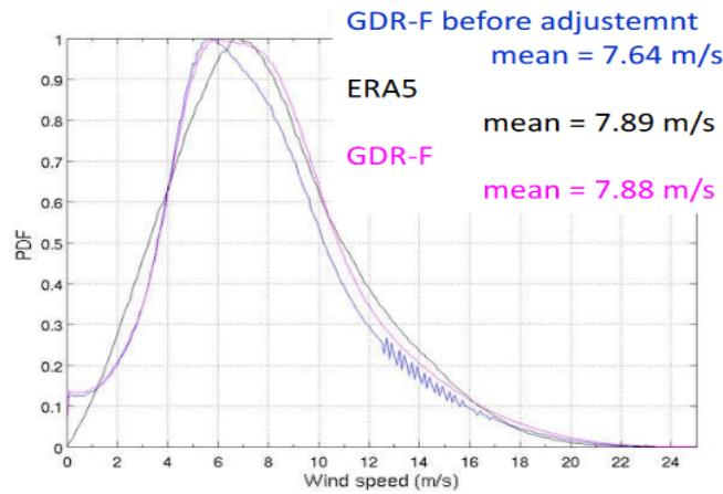
Figure 43 – Wind speed comparison product and ERA5 model
