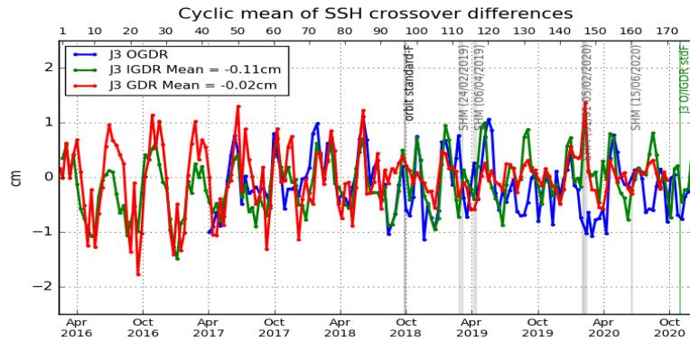
Figure 4 – Monitoring of mean of Jason-3 SSH crossover differences for OGDRs, IGDRs and GDRs. Only data with  $|\text{latitude}| < 50^\circ$ , bathymetry  $< -1000\text{m}$  and low oceanic variability were selected. (ocean\_tide\_sol1 = GOT is used in SSH computation)
