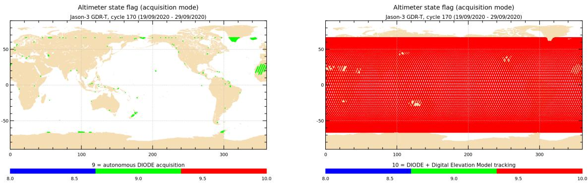
*Figure 2 – Acquisition mode for cycle 170 (identical to acquisition mode automatic switch for cycles 169-177). Left: 9 = autonomous DIODE acquisition / tracking. Right: 10 = DIODE + Digital Elevation Model tracking*
