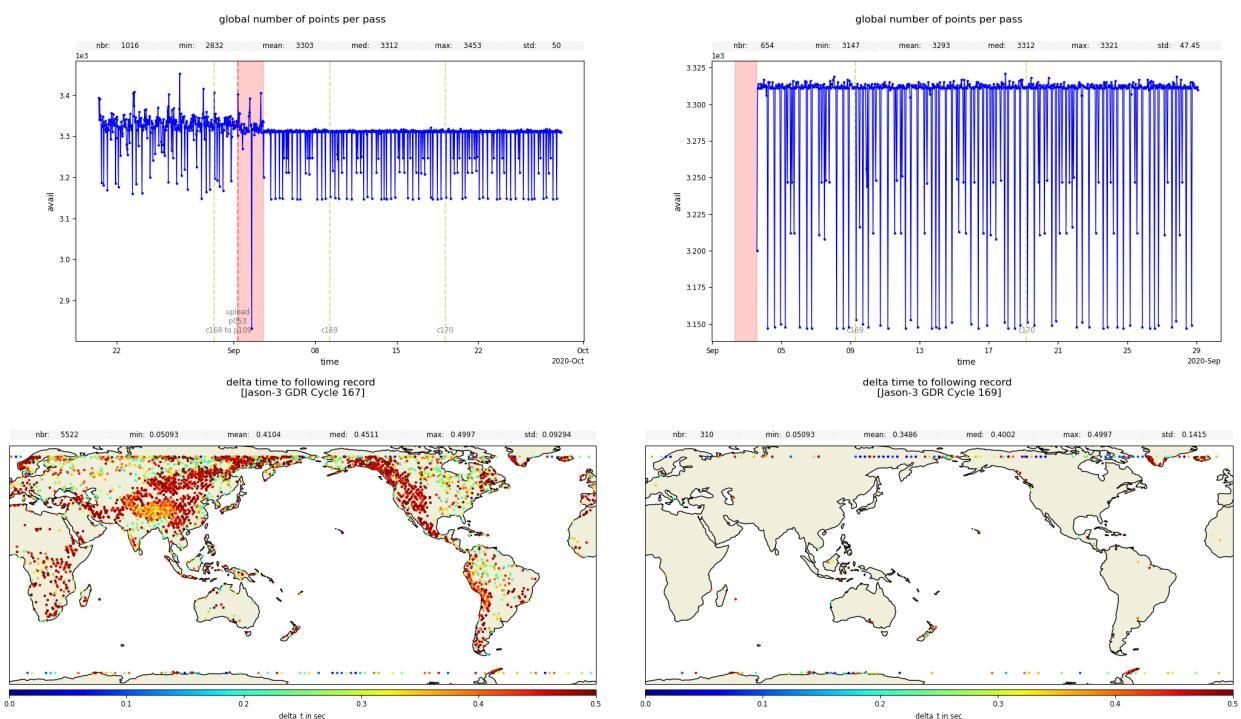
**Figure 63 – Top:** Number of records per pass for dataset at 1Hz **Left:** before, during, and after update **Right:** after update only **Bottom:** Map of points with difference between two consecutive points at 1Hz < 0.5s before update on the left, and after update on the right
