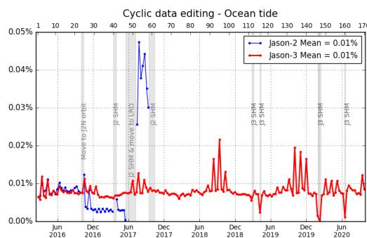
Figure 18 – Percentage of edited measurements by ocean tide threshold criterion. Cycle per cycle monitoring compared with Jason-2.
