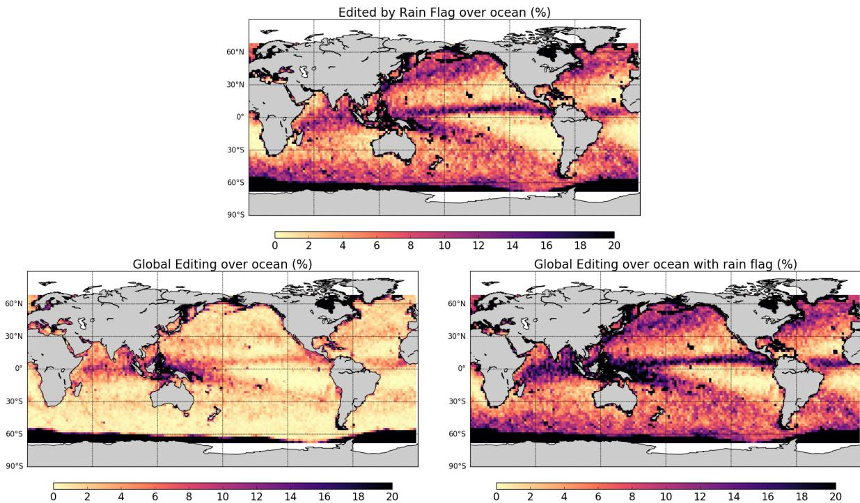
*Figure 9 – Top: Percentage of edited measurements by altimeter rain flag criterion. Bottom left: Map of global edited measurements without considering the rain flag. Bottom right: Map of global edited measurements using all criteria and considering the rain flag. All figures are computed over ocean and from cycle 134 to 170.*
