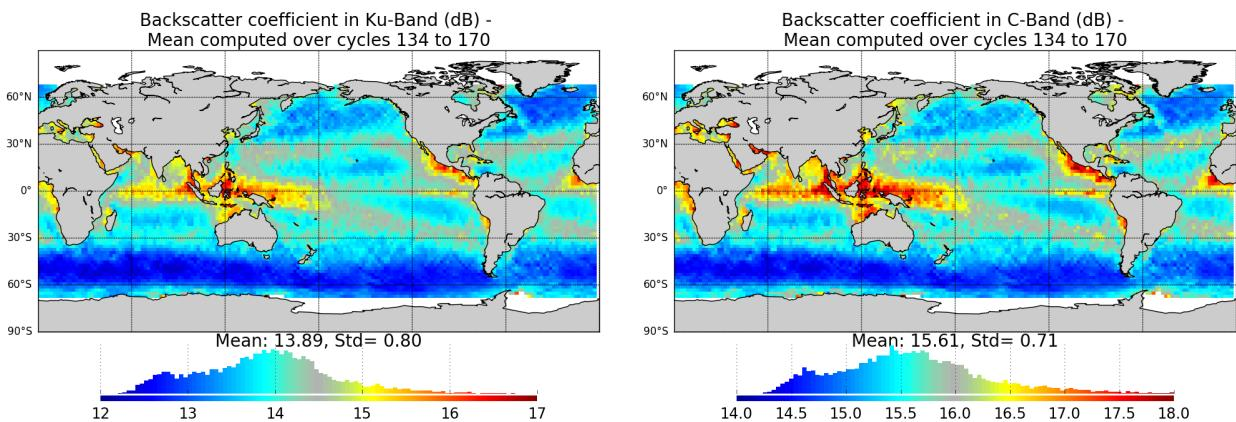
**Figure 31 –** Map of backscatter coefficient for Jason-3 averaged over cycles 134 to 170, in Ku-band (left) and in C-band (right).
