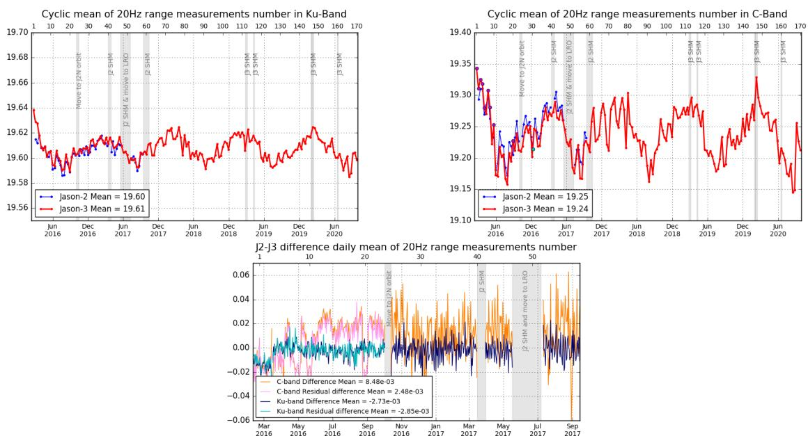
*Figure 22 – Top:* Cyclic monitoring of number of elementary 20 Hz range measurements for Jason-2 and Jason-3 for Ku-band and C-band. *Bottom:* Jason-2 - Jason-3 difference daily monitoring of elementary 20 Hz range measurements number (until september 2017).
