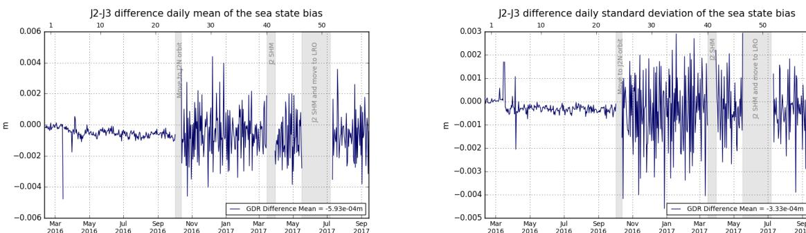
Figure 46 – Jason-2 - Jason-3 difference daily monitoring of the sea state bias mean (left) and standard deviation (right).
