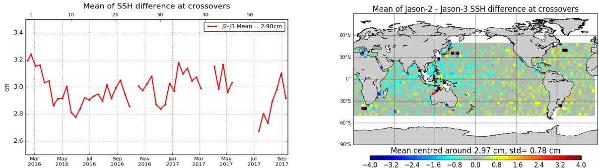
*Figure 6 – Cyclic monitoring of Jason-2 - Jason-3 SSH crossover differences mean (left) and map over cycle 1 to 58 (right). Only data with  $|latitude| < 50^\circ$ , bathymetry  $< -1000m$  and low oceanic variability were selected.*
