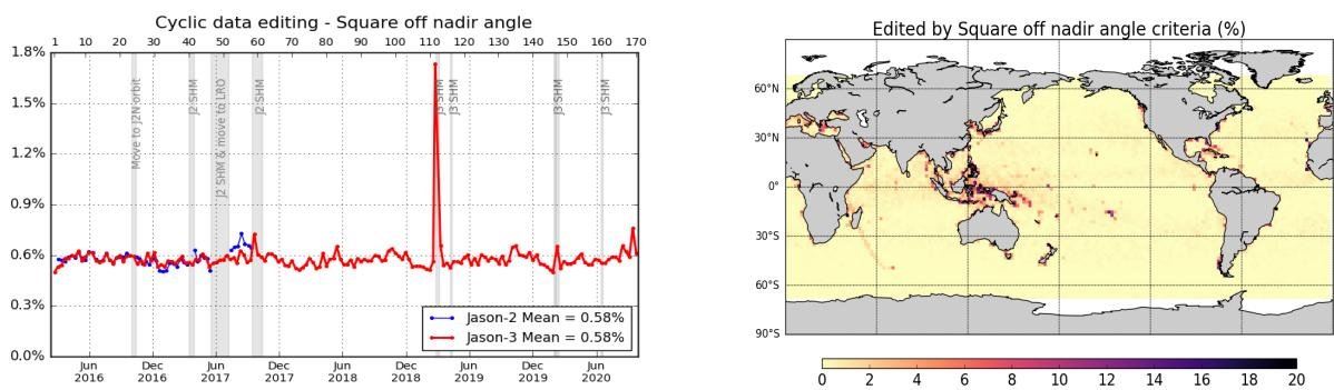
Figure 19 – Percentage of edited measurements by square off nadir angle threshold criterion. Left: Cycle per cycle monitoring compared with Jason-2. Right: Jason-3 averaged map from cycle 134 to 170.
