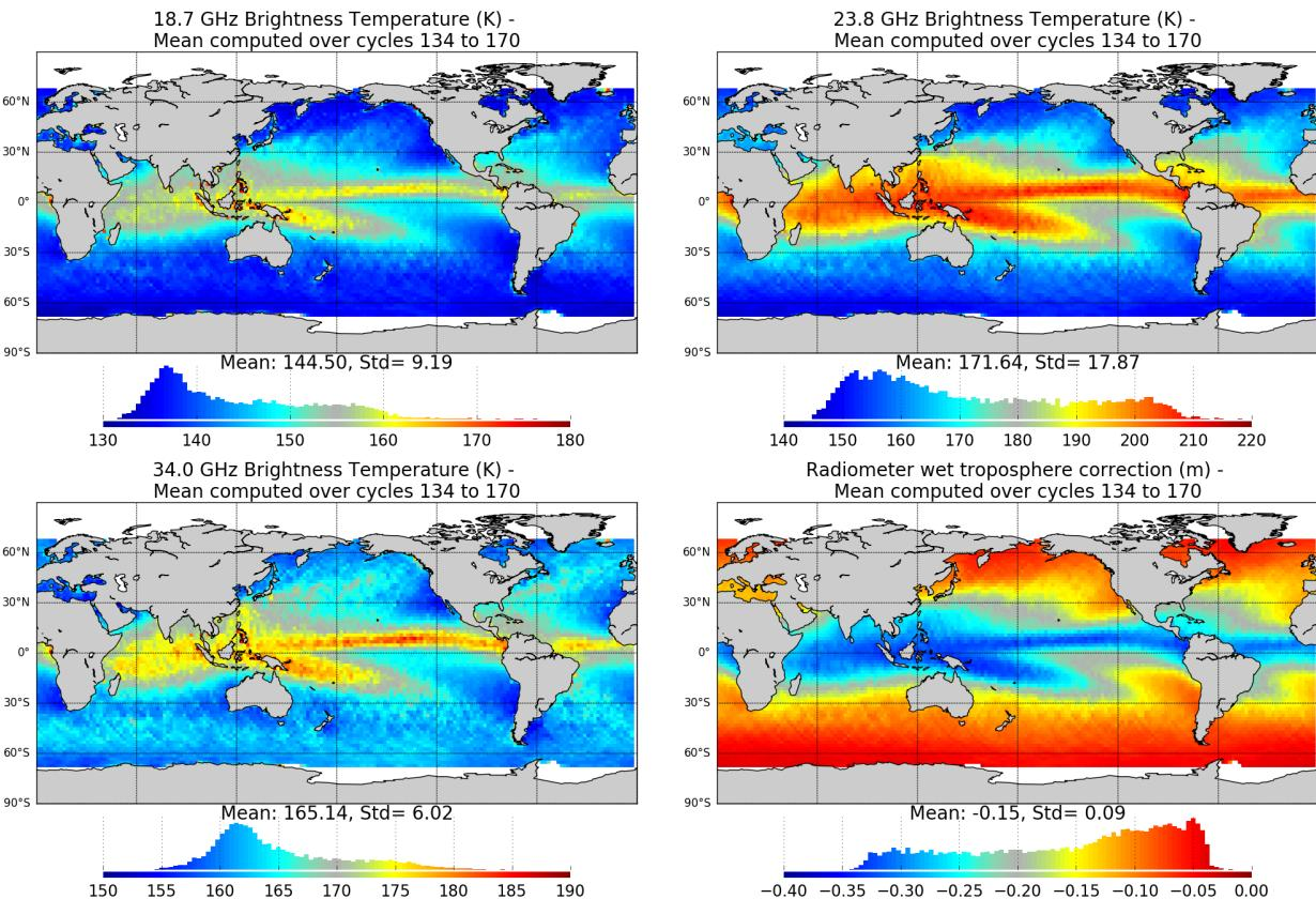
Figure 38 – Map of Jason-3 brightness temperatures averaged over cycles 134 to 170: 18.7 Ghz channel (top left), 23.8 Ghz channel (top right) and 34.0 Ghz channel (bottom left). Map of AMR wet troposphere correction for Jason-3 averaged over cycles 134 to 170 (bottom right)
