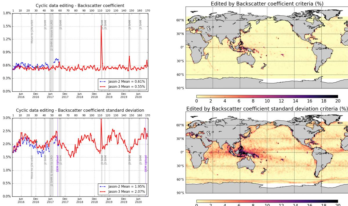
*Figure 13 – Percentage of edited measurements by backscatter coefficient threshold criterion (top) and by 20Hz backscatter coefficient standard deviation threshold criteria (bottom). Cycle per cycle monitoring compared with Jason-2 (left, Jason-2 DEM cycle in cyan. Jason-3 median tracker cycles in purple) and Jason-3 averaged map from cycle 134 to 170 (right).*
