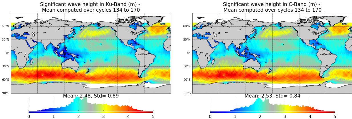
Figure 34 – Map of significant wave height for Jason-3 averaged over cycles 134 to 170, in Ku-band (left) and in C-band (right).
