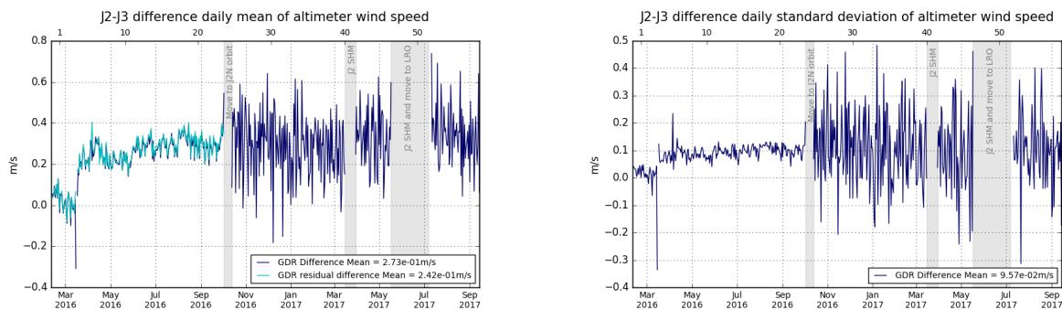
Figure 42 – Jason-2 - Jason-3 difference daily monitoring of altimeter wind speed mean (left) and standard deviation (right).
