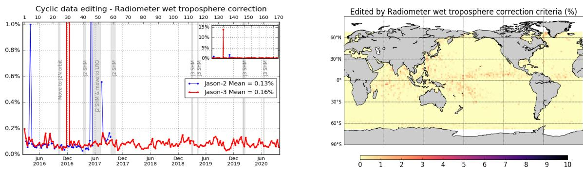
*Figure 14 – Percentage of edited measurements by radiometer wet troposphere correction threshold criterion. Left: Cycle per cycle monitoring compared with Jason-2. Right: Jason-3 averaged map from cycle 134 to 170.*
