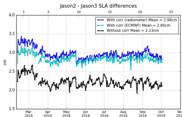
Figure 52 – Daily monitoring of SSH bias between Jason-2 and Jason-3 before Jason-2 moved to interleaved ground-track in October 2016: SSH bias without applying geophysical corrections (**black**) and with corrections using radiometer wet troposphere correction (**blue**) or using ECMWF model wet troposphere correction (**cyan**).
