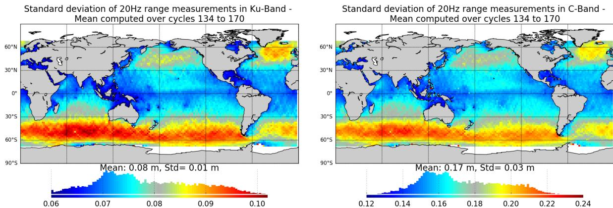
**Figure 25 –** Map of 20 Hz range measurements standard deviation for Jason-3 averaged over cycles 134 to 170, in Ku-band (left) and in C-band (right).
