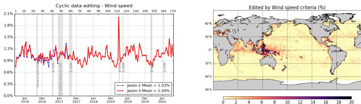
Figure 16 – Percentage of edited measurements by wind speed threshold criterion. Left: Cycle per cycle monitoring compared with Jason-2. Right: Jason-3 averaged map from cycle 134 to 170.
