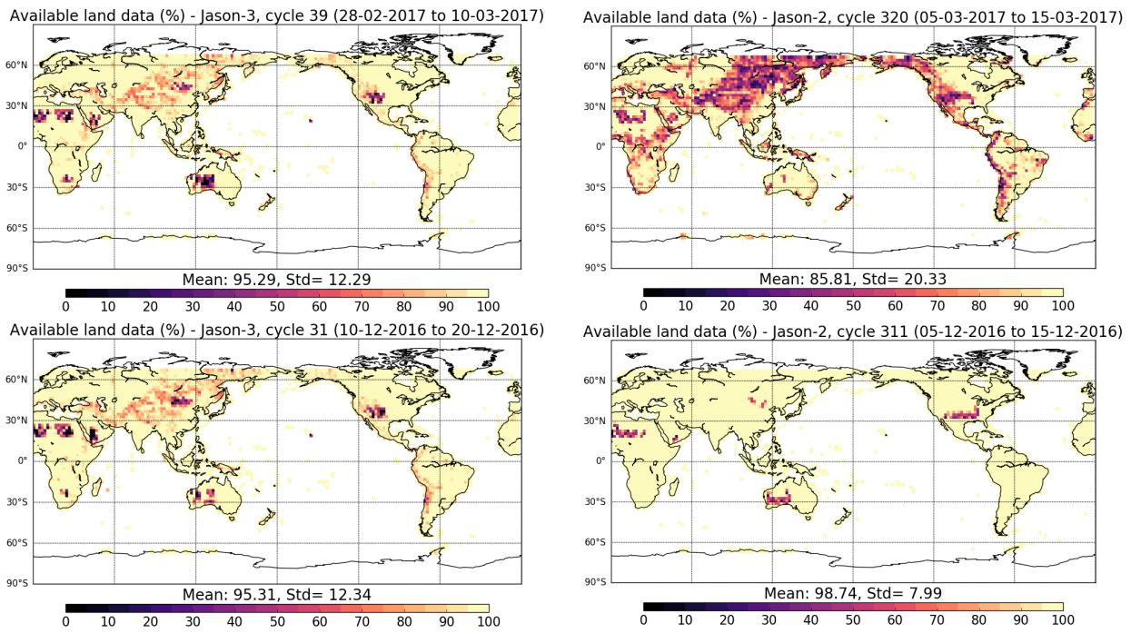
*Figure 4 – Map of percentage of available measurements over land for Jason-3 (left) and for Jason-2 (right). Top: Jason-3 cycle 039 in DEM mode and Jason-2 cycle 320 in median mode. Bottom: Jason-3 cycle 031 in DEM mode and Jason-2 cycle 311 in DEM mode*
