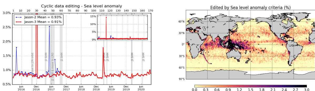
*Figure 21 – Percentage of edited measurements by sea level anomaly threshold criterion. Left: Cycle per cycle monitoring compared with Jason-2. Right: Jason-3 averaged map from cycle 134 to 170.*
