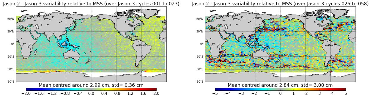
*Figure 53 – GDR data. Caution: color map ranges are different between the two figures. Left: Map of SLA difference between Jason-2 and Jason-3 over tandem phase Right: Map of Jason-2 and Jason-3 SLA differences for Jason-3 cycles 025 to 058*
