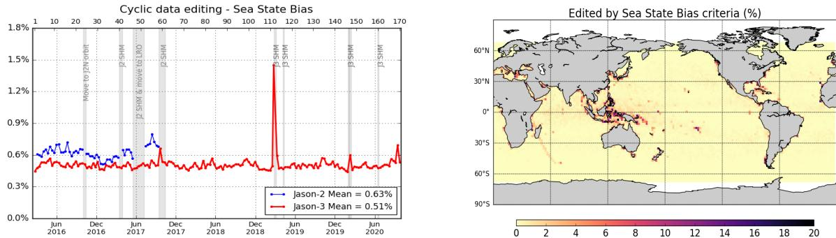
Figure 17 – Percentage of edited measurements by sea state bias threshold criterion. Left: Cycle per cycle monitoring compared with Jason-2. Right: Jason-3 averaged map from cycle 134 to 170.
