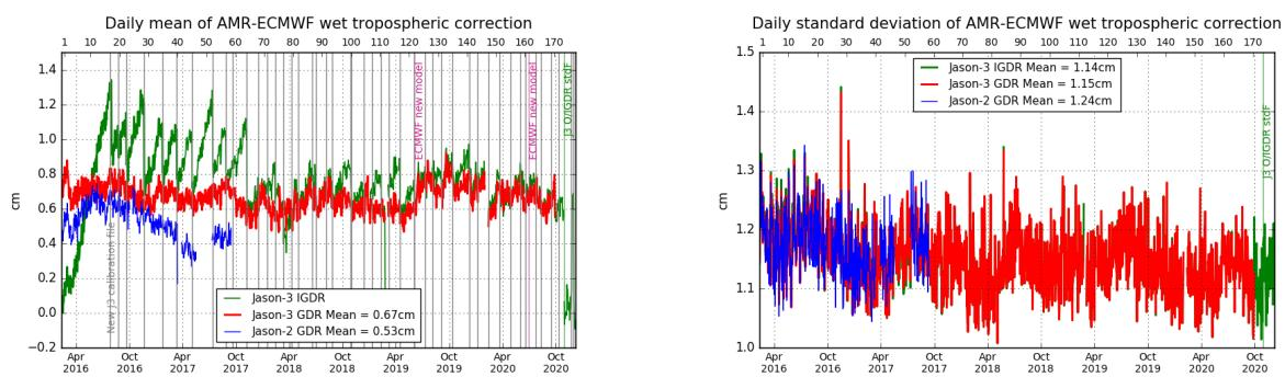
Figure 40 – Daily monitoring of AMR minus ECMWF model wet tropospheric correction. mean (left) and standard deviation (right)
