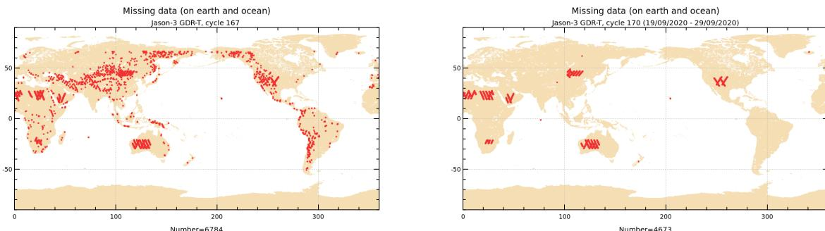
Figure 62 – Map of missing data over land and ocean. Left: before update (cycle 167) Right: after update (cycle 170).
