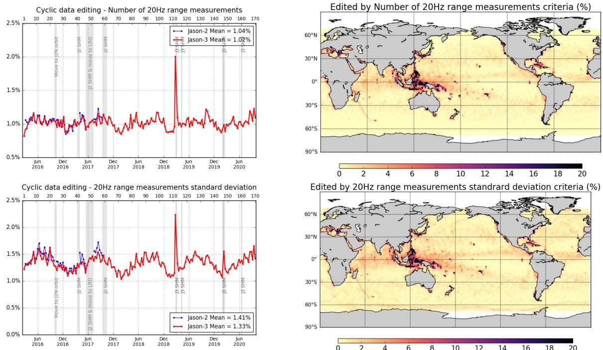
Figure 11 – Percentage of edited measurements by 20Hz range measurements threshold criterion (top) and by 20Hz range measurements standard deviation threshold criteria (bottom). Cycle per cycle monitoring compared with Jason-2 (left) and Jason-3 averaged map from cycle 134 to 170 (right).
