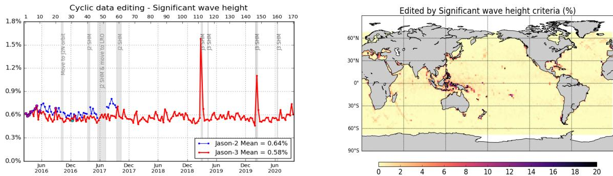
*Figure 12 – Percentage of edited measurements by SWH threshold criterion. Left: Cycle per cycle monitoring compared with Jason-2 (Jason-2 DEM cycle in cyan. Jason-3 median tracker cycles in purple.) Right: Jason-3 averaged map from cycle 134 to 170 .*
