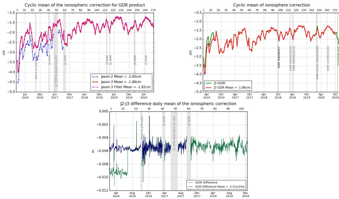
Figure 35 – Cyclic monitoring of ionospheric correction for Jason-2 and Jason-3. (left). Cyclic monitoring of Jason-3 ionospheric correction for IGDR and GDR data (right). Jason-2 - Jason-3 difference daily monitoring of ionospheric correction (bottom).
