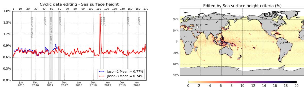
Figure 20 – Percentage of edited measurements by sea surface height threshold criterion. Left: Cycle per cycle monitoring compared with Jason-2. Right: Jason-3 averaged map from cycle 134 to 170.
