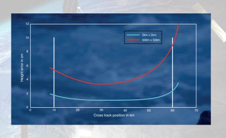
Level 2 products have a resolution of 2 km by 2 km. If each swath is 58 km wide, data quality is degraded at the edges. The error due to instrument noise is still less than 2 cm between 10 and 60 km.
